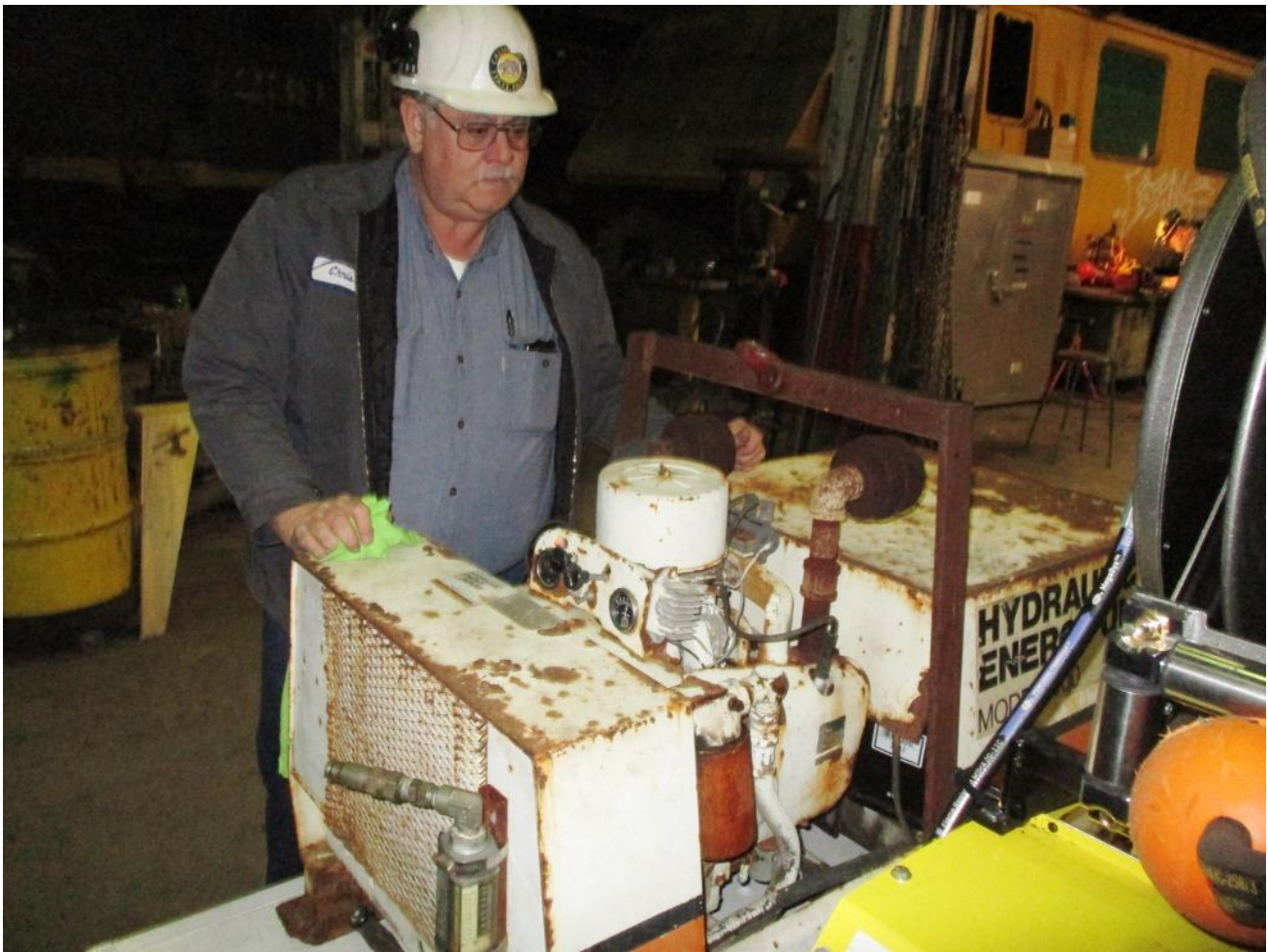
Chris C. assesses the issues with the old hydraulic power unit
